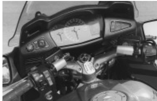
Left: The speedo and tach are easy to read, but the LCD displays aren't. Note the lower surface of the dash, which looks to be ready for speakers. But efforts to contain the heat from reaching the rider have made the fairing compartments very hot in warm weather.
