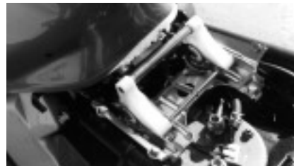
Above: Seat adjustment mechanism allows three positions, from 30.5" to 31.75".
