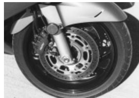
Below: The brakes are much more powerful than the ST1100's but we found the brake pads too progressive. The Linked Braking System is carried over, but with less "bias" than before.
